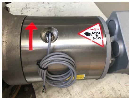
Figure 5.57: Zero speed indicator (on coupling)
