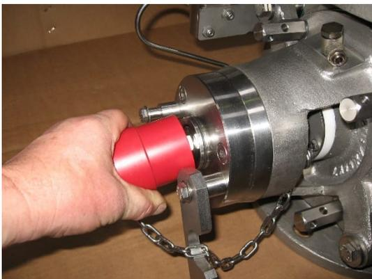
Loosen nut from locking unit (180) and remove.
