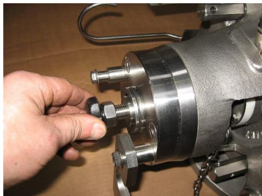
Secure nut with minimum force, if possible, prevent rotor to rotate.
