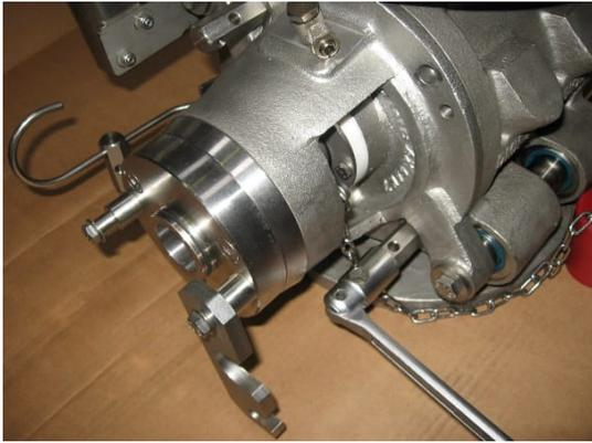
If necessary two bolts can be fitted into jacking holes of cover to enable dismantling.
