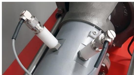
Figure 5.63: Rotor pick-ups for rotor interference detection
