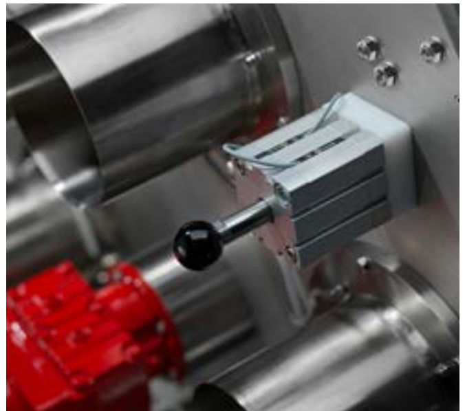
Exact alignment between ports and internal swan neck.
